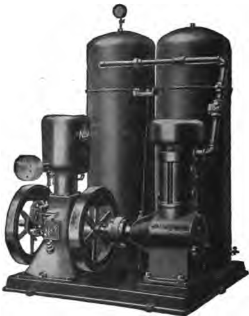
FIG. 176.—Gas Engine with an Air Compressing Outfit. Used for compressing air in a garage. The two large tanks or receivers in the rear are for storing the compressed air. A gauge is on top of the tank to indicate the pressure in the tank.
